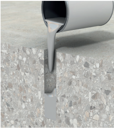
Mix and pour grout/resin into hole.
